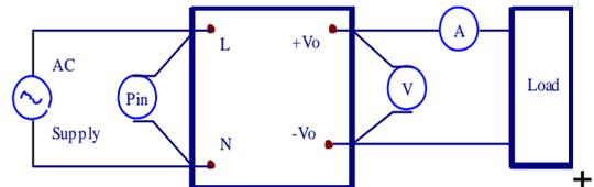
Figure 1 TRG36 VI Series Test Setup
