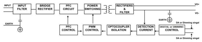
Figure 1. Electrical Block Diagram
