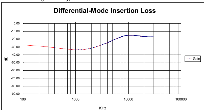
Figure 3. Typical Differential-Mode Insertion Loss
