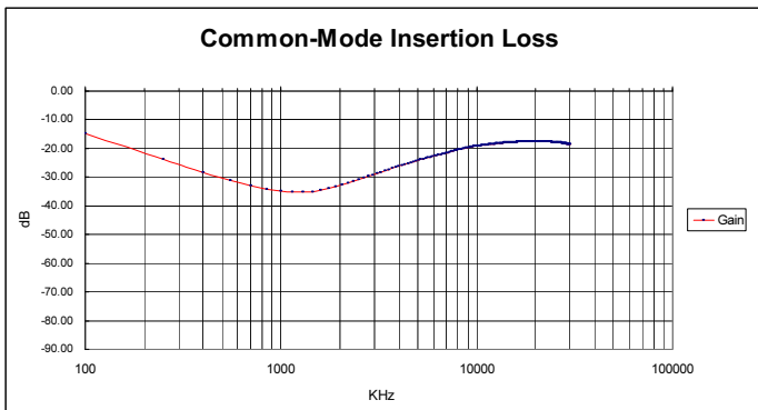
Figure 2. Typical Common-Mode Insertion Loss
