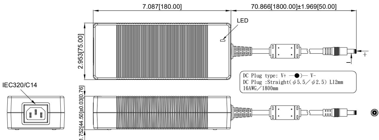
\* For Output Voltage 12Vdc and 24V model, it must select Din Power Plug Molded Type or equivalent
