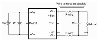
If the remote sense feature is not to be used, the sense pins should be connected locally. The +Sense pin should be connected to the +Vout pin at the module and the -Sense pin should be connected to
