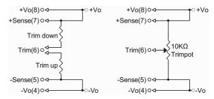
In order to trim the voltage up or down, one needs to connect the trim resistor either between the trim pin and -Sense for trim-up or between trim pin and +Sense for trim-down. The output voltage trim range is -20% to +15%. This is shown:
