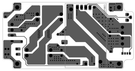
Figure3 PCB layout bottom view
