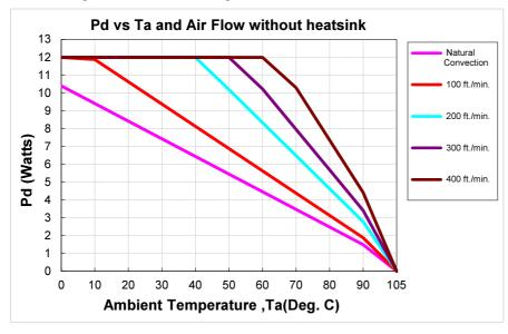
The following curve is the de-rating curve of CQB75W8 series without heat sink.
