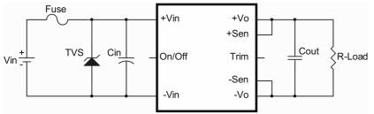
The external input capacitor (Cin) and transient voltage suppressor diode (TVS) are required if CQB75W8 series has to meet EN61000-4-4, EN61000-4-5.
