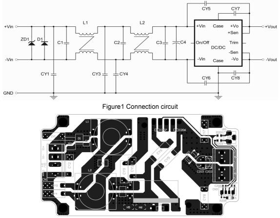
Figure2 PCB layout top view
